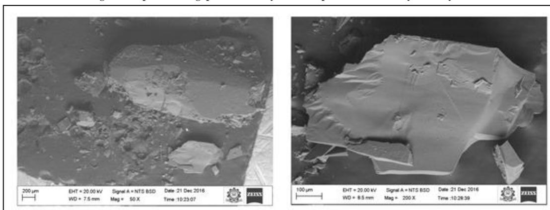
Figure 8: SEM photograph for 4-carboxyanilinium perchlorate monohydrate crystal
