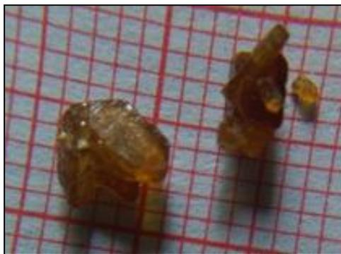
Figure 1: Grown crystal of 4-carboxyanilinium perchlorate monohydrate
