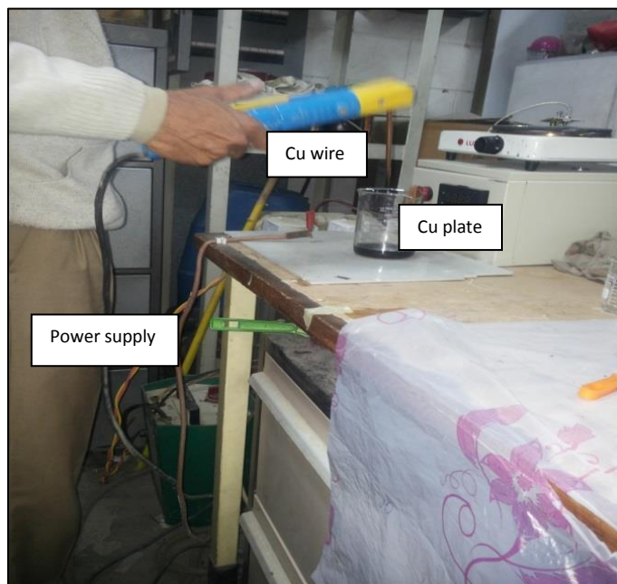
Figure 1: The exploding wire system used to synthesizing the pure CuI nanoparticles
