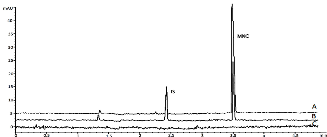
Figure 2: MEKC electropherogram: (A) MNC hydrochloride RS; (B) MNC capsules; (C) Placebo solution
