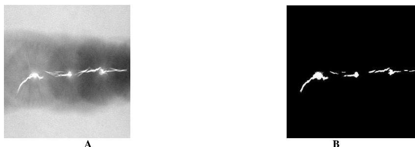
Fig.5: A) the image showing the welding defects B) connectivity analysis results on seed point 8
