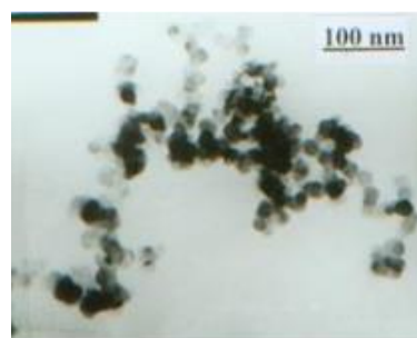
Fig.2 TEM photograph of Ce_2(C_4H_4O_4)_3 nanocrystallites (synthesized according to No.16 in Table 2)
