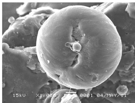
Figure 8. Result of SEM of empty polycaprolactone microcapsules with 1000 times magnification
