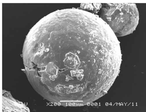
Figure 11. Result of SEM of Formula 3 of 2,4-D microcapsules with 200 times magnification
