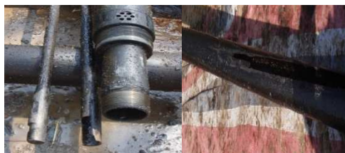
Fig.10 worn column before optimization
