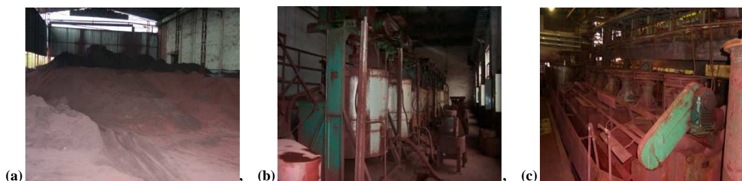
Fig.1 Diagram of (a) raw pyrite cinder and (b) industrial scale steel stirred mill and (c) BF-1.2 XFG cell
