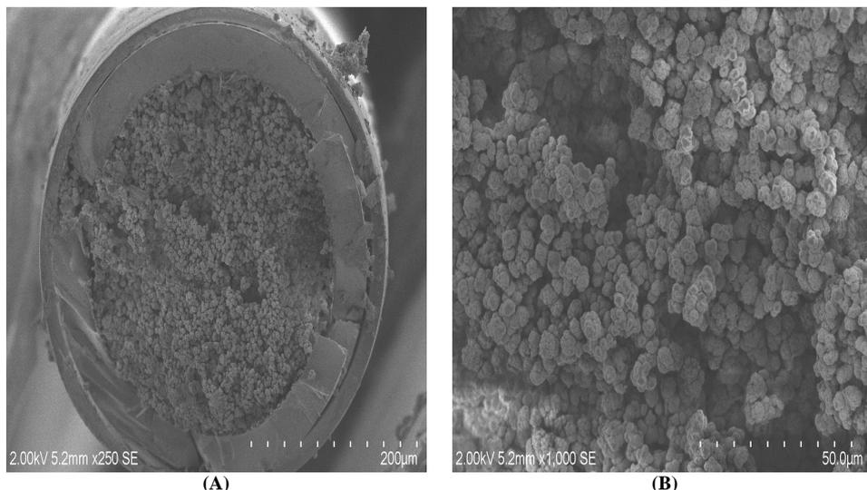
**Figure 1.** Scanning Electron Microphotograph of monolith column (A) 250x (B) 1000x
