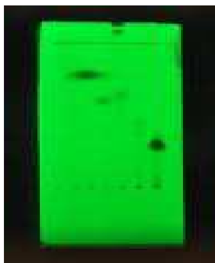
Figure 4: TLC chromatogram of Berberine isolated from Berberis aristata was viewed under UV light
