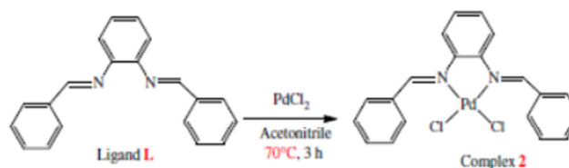
Scheme 7: complex formation of Ligand L in the presence of PdCl 2 and Acetonitrile
