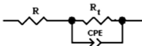
Figure 4: The equivalent circuit of the impedance spectra obtained for of Salvia officinalis extract
