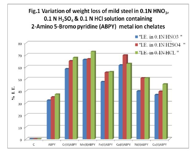
The use of inhibitors is one of the most practical methods for protection against corrosion. To study inhibition efficiency the 2-Amino 5-Bromo pyridine (ABPY) and their metal ion chelates are used on mild steel in different acidic solution. Corrosion inhibition effect of 2-Amino 5-Bromo Pyridine(ABPY) metal ion chelates on mild steel in different acidic media 0.1N  $HNO_3$ , 0.1N  $H_2SO_4$  and 0.1 N HCl solution has been assessed using weight loss technique.
