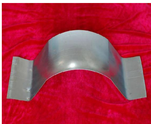
Fig.11 The spherical parts formed by MRSF prototype
