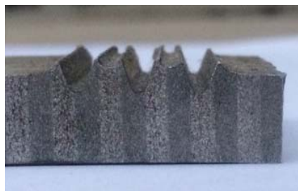
Fig. 16 The test results of hard aluminum cold roll-beating
