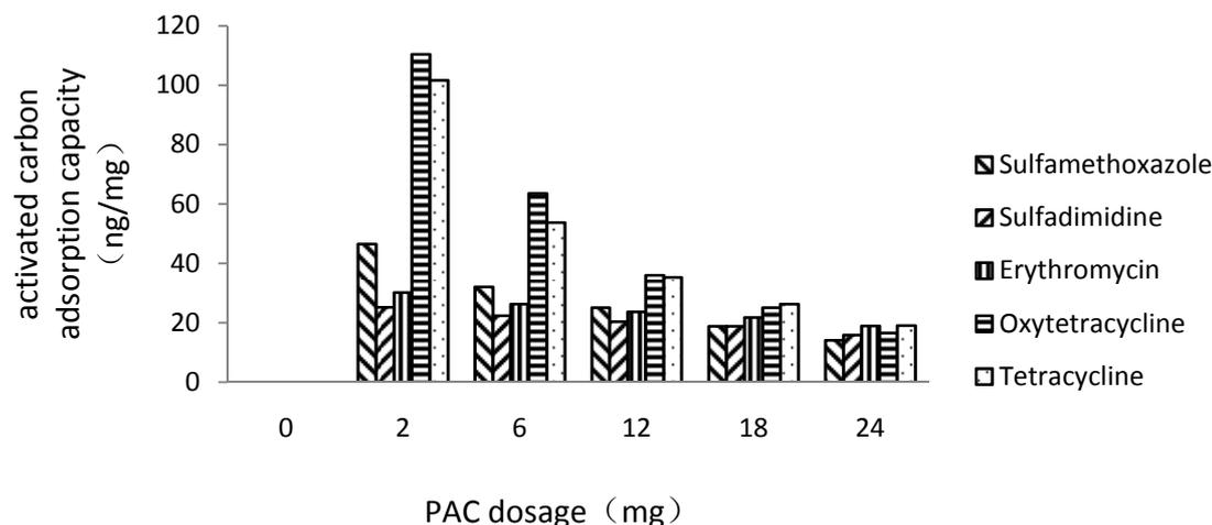
Fig.4 PAC adsorption capacity of the typical antibiotics
