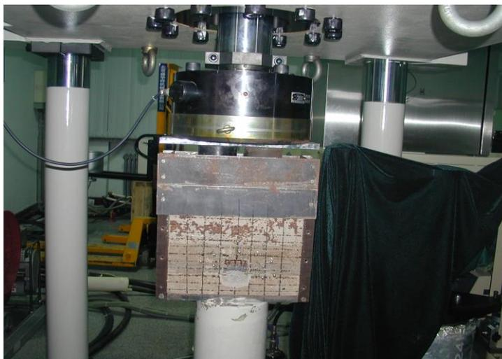
Fig.1: TIR detection during uniaxial loading of the bolted roadway samples
