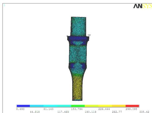
**Fig.2 Mises stress nephogram of sucker rod**
