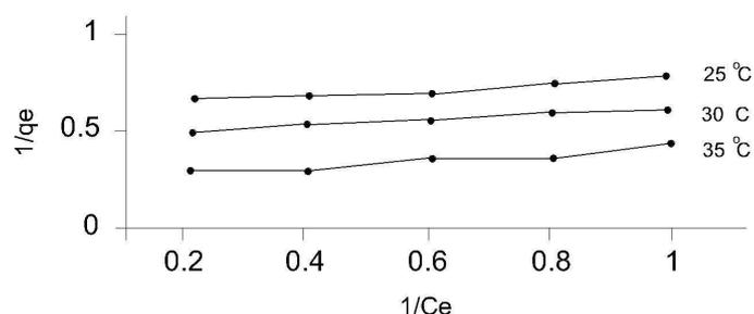
**Fig. 4. Langmuir plots for the adsorption of chrom Red-B onto diatomite**
