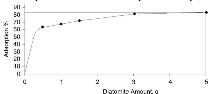
Fig. 2. Chrome Red-B dye of adsorption by different amount of diatomite (30 °C, 195 rpm, 8h.)
