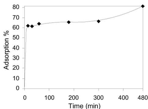
Fig.3. Chrome Red-B dye of adsorption on diatomite for different times (3 g diatomite, 30 °C, 195 rpm)
