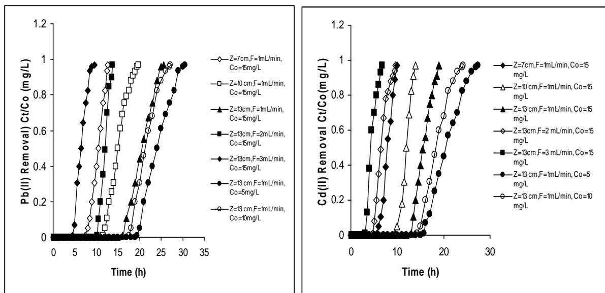
Fig.2 Breakthrough curve for Pb(II) sorption: Z= 7,10 and 13 cm, F=1,2 and 3 mL/min and  $C_o=5, 10$  and 15mg/L, pH = 5, temp. =  $\pm 28^\circ\text{C}$
