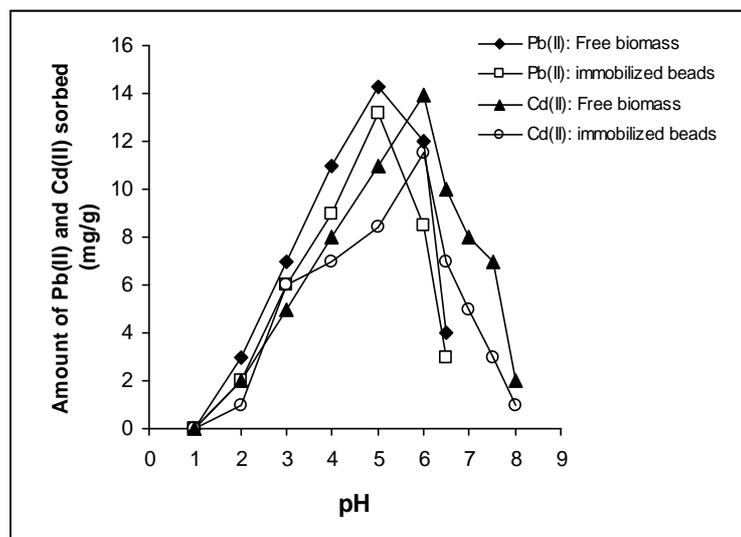
Fig. 1 Effect of pH: pH range= 1 to 6.5 for Pb(II) and 1 to 8.0 for Cd(II),  $C_0=15$  mg/L, room temp. =  $\pm 28^\circ\text{C}$
