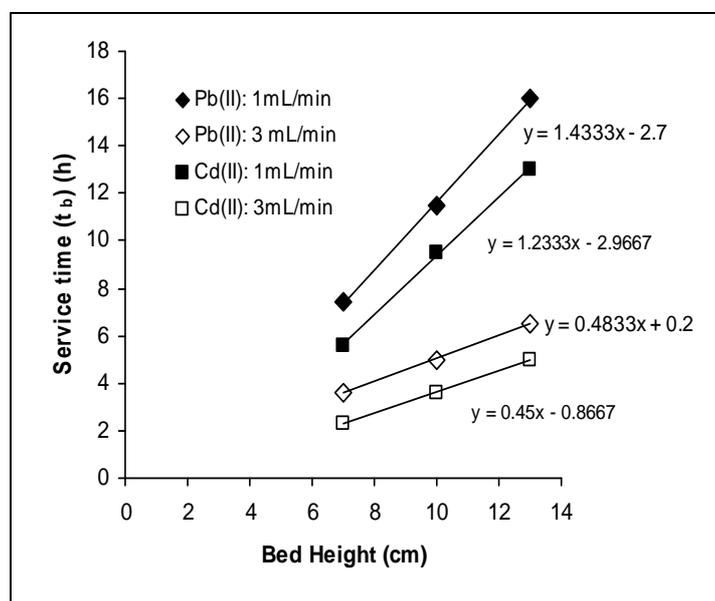
Fig. 4 Bed Depth Service Time (BDST) Plot
