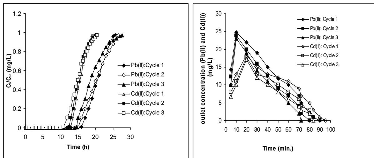
Fig. 5(a) Sorption breakthrough curve for Pb(II) and Cd(II) during three sorption cycle:  $F = 1 \text{ mL/min}$ ,  $C_0 = 15 \text{ mg/L}$ ,  $Z = 25 \text{ cm}$
