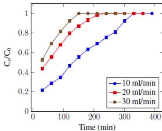
Figure 3: Breakthrough curves for Cadmium at 100 g bed weight, IMC =100 ppm at different flow rates of 10, 20 and 30 ml/min
