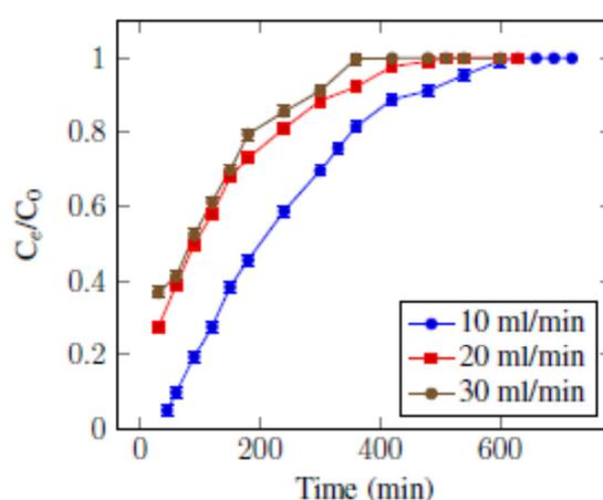
Figure 7: Breakthrough curves for Copper at 150 g bed weight, IMC =100 ppm at different flow rates of 10, 20 and 30 ml/min
