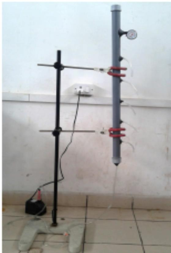
Fig 1 Experimental setup of Continuous flow column
