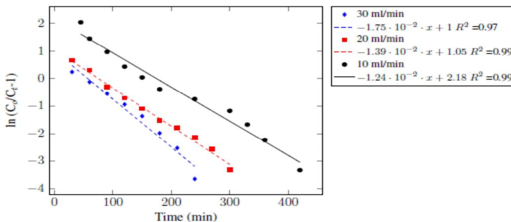
Figure 9: Thomas model for Cd (II) at 150 g bed weight and at different flow rates
