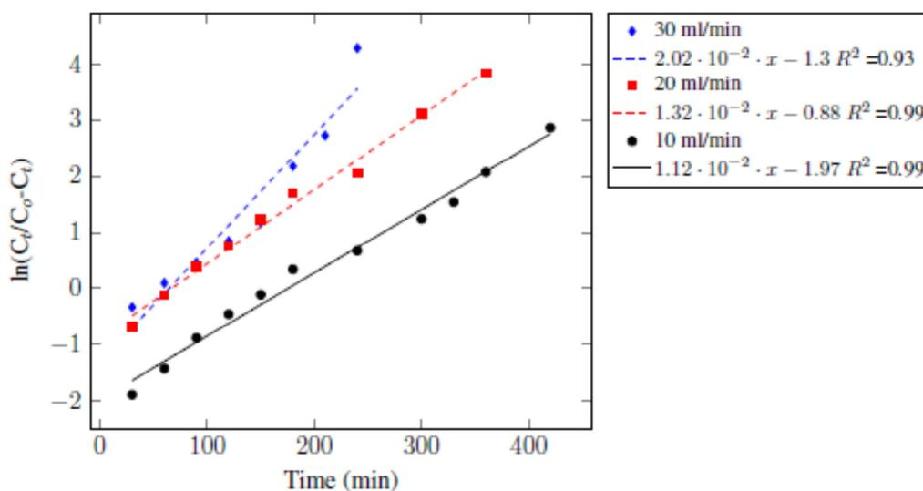
Figure 10: Yoon- Nelson model for Cu (II) at 100 g of bed weight and different flowrates
