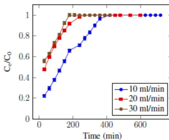
Figure 5: Breakthrough curves for Copper at 50 g bed weight, IMC =100 ppm at different flow rates of 10, 20 and 30 ml/min
