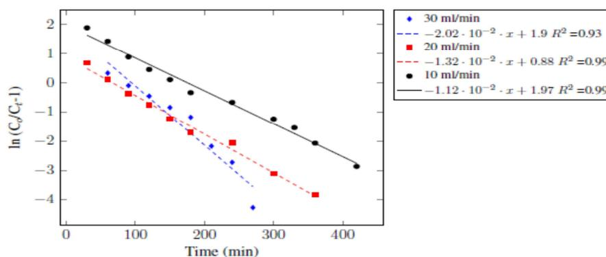
Figure 8: Thomas model for Cu (II) at 100 g bed weight and at different flow rates
