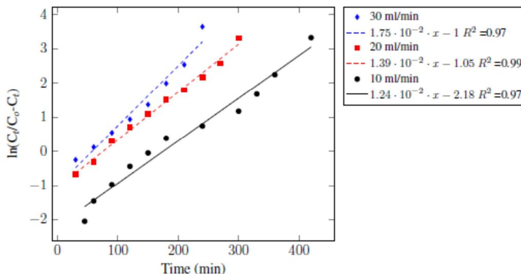
Figure 11: Yoon- Nelson model for Cd (II) at 150 g of bed weight and different flow rates
