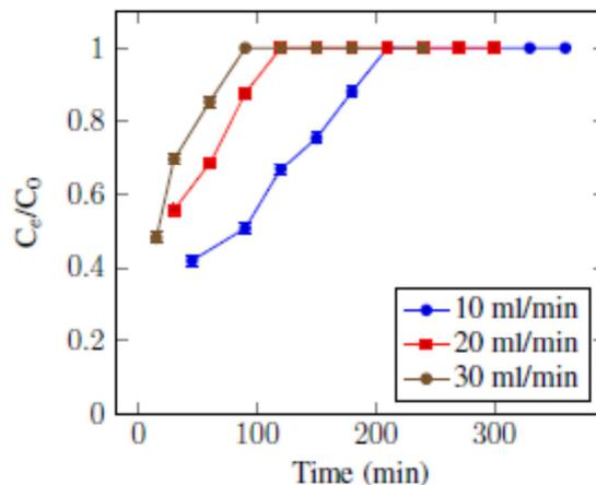
Figure 2: Breakthrough curves for Cadmium at 50 g bed weight, IMC =100 ppm at different flow rates of 10, 20 and 30 ml/min
