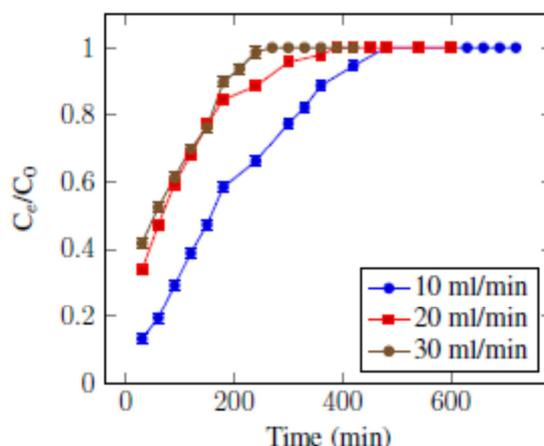
Figure 6: Breakthrough curves for Copper at 100 g bed weight, IMC =100 ppm at different flow rates of 10, 20 and 30 ml/min
