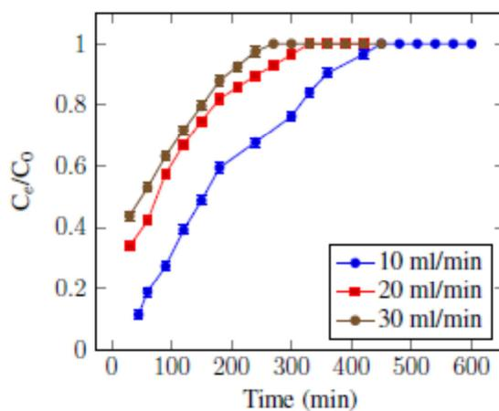
Figure 4: Breakthrough curves for Cadmium at 150 g bed weight, IMC =100 ppm at different flow rates of 10, 20 and 30 ml/min
