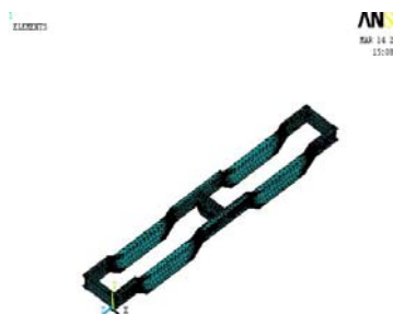
Fig.4: The finite element model mode of the chassis frame
