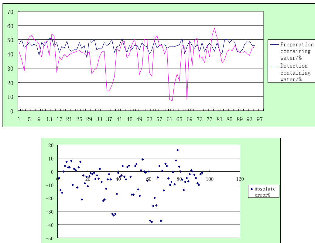
Fig. 3 The year 2007discrete distribution maps of absolute error comparative data(95 basic laboratories data)
