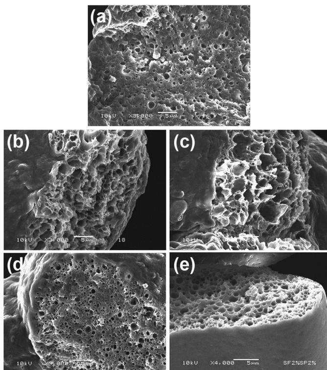
**Fig. 3.** SEM micrographs of fractured microparticles prepared with SS/SF blend ratios of (a) 100/0, (b) 75/25, (c) 50/50, (d) 25/75 and (e) 0/100 (w/w). All bars = 5  $\mu$ m
