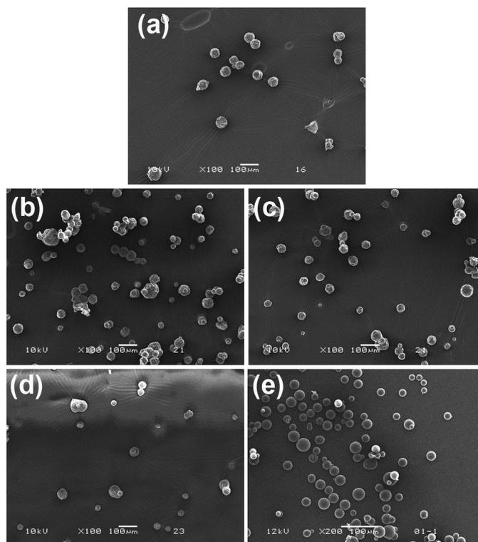
**Fig. 1. SEM micrographs of blend microparticles prepared with SS/SF blend ratios of (a) 100/0, (b) 75/25, (c) 50/50, (d) 25/75 and (e) 0/100 (w/w). All bars = 100  $\mu\text{m}$**
