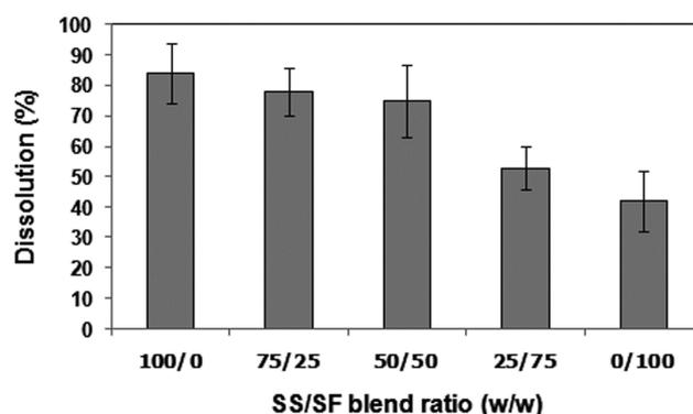
Fig. 5. Dissolution of blend microparticles prepared with different SS/SF blend ratios
