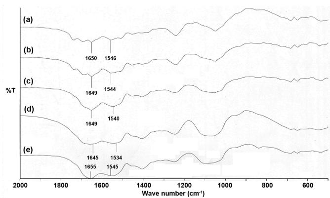
Fig. 4. FTIR spectra of blend microparticles prepared with SS/SF blend ratios of (a) 100/0, (b) 75/25, (c) 50/50, (d) 25/75 and (e) 0/100 (w/w)
