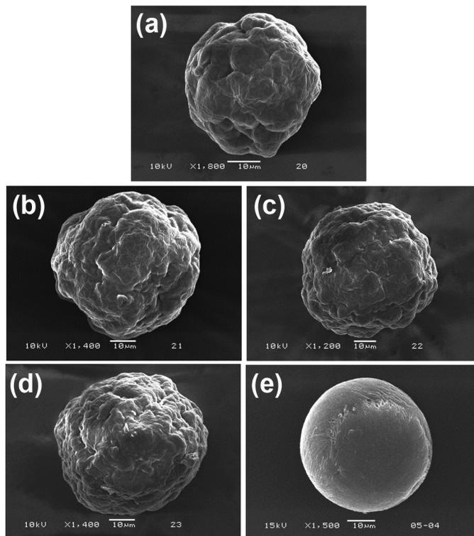
**Fig. 2.** Expanded SEM micrographs of blend microparticles prepared with SS/SF blend ratios of (a) 100/0, (b) 75/25, (c) 50/50, (d) 25/75 and (e) 0/100 (w/w). All bars = 10  $\mu$ m
