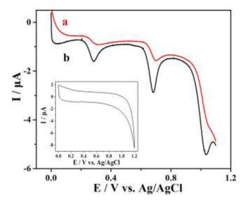
Fig. 2 LSVs of bare GCE (a), PCA/GCE (b), in pH 6.5 PBS containing 20 μM UA, 40μM XA and 80 μM HX with a scan rate of 50 mV s<sup>-1</sup>. Inset: CV of PCA/GCE in pH 6.5 PBS
