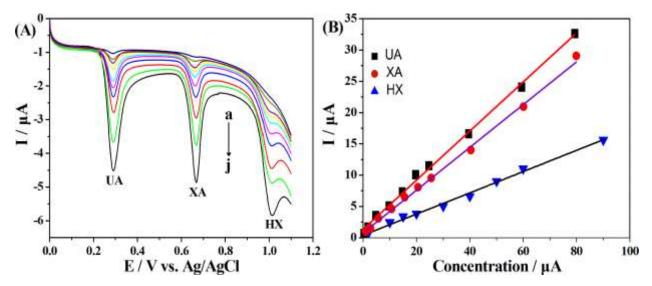
Fig. 6 (A) LSV of different concentrations of UA, XA (a-j: 0.2, 2, 5, 10, 15, 20, 25, 40, 60, 80 μM) and HX (a-j: 0.5, 2, 10, 15, 20, 30, 40, 50, 60, 90 μM) on PCA/GCE in pH 6.5 PBS. (B) Concentration calibration curve of the LSV current response for UA, XA and HX
