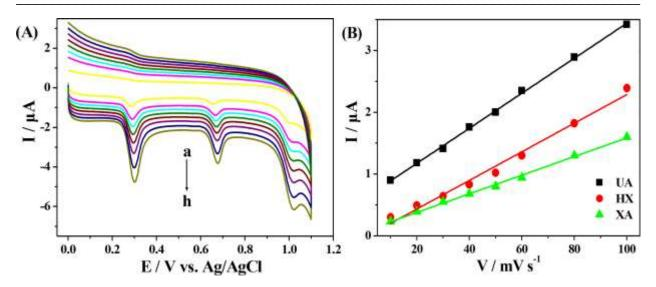
Fig. 3 (A) CVs of 50 μM UA, 25μM XA and 50μM HX mixture solution on PCA/GCE at with different scan rates (a-h: 10, 20, 30, 40, 50, 60, 80, 100 mV s<sup>-1</sup>) in pH 6.5 PBS. (B) Plots of the oxidation peak current versus the scan rate
