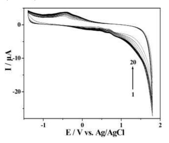
Fig. 1 CV of CA in electropolymerization process from 1 to 20 cycles. CA:  $2.5 \times 10^{-3}$  M; supporting electrolyte: pH 7.4 PBS containing 0.01 M KNO<sub>3</sub>; scan rate: 100 mV s<sup>-1</sup>
