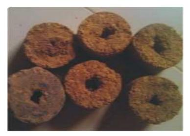
Plate 2: Bambaranut shell briquettes produced
