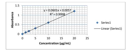
Figure 2: Calibration curve of ofloxacin pure sample
