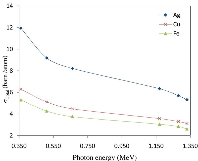
Fig 5 Plots of total photon attenuation coefficient ( $\sigma_{\text{total}}$ ) v/s photon energy (MeV) for Ag, Cu and Fe (0.2 cm collimation)
