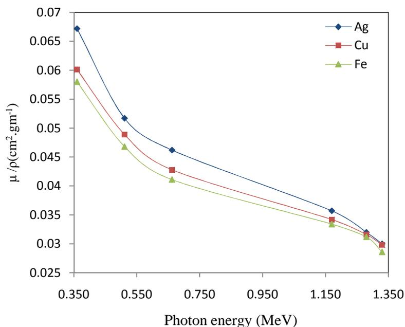
**Fig 4 Plots of photon attenuation coefficient ( $\mu/\rho$ ) v/s photon energy (MeV) for Ag, Cu and Fe (0.2 cm collimation)**
