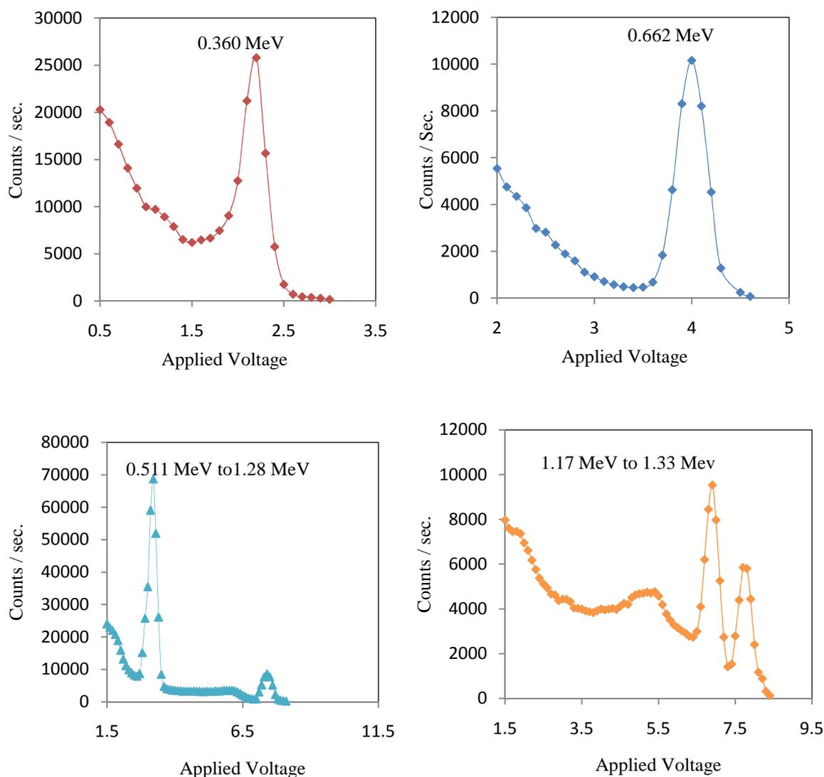
**Fig.2 Gamma spectra of Ba<sup>133</sup>, Cs<sup>137</sup>, Na<sup>22</sup>, and Co<sup>60</sup>**
