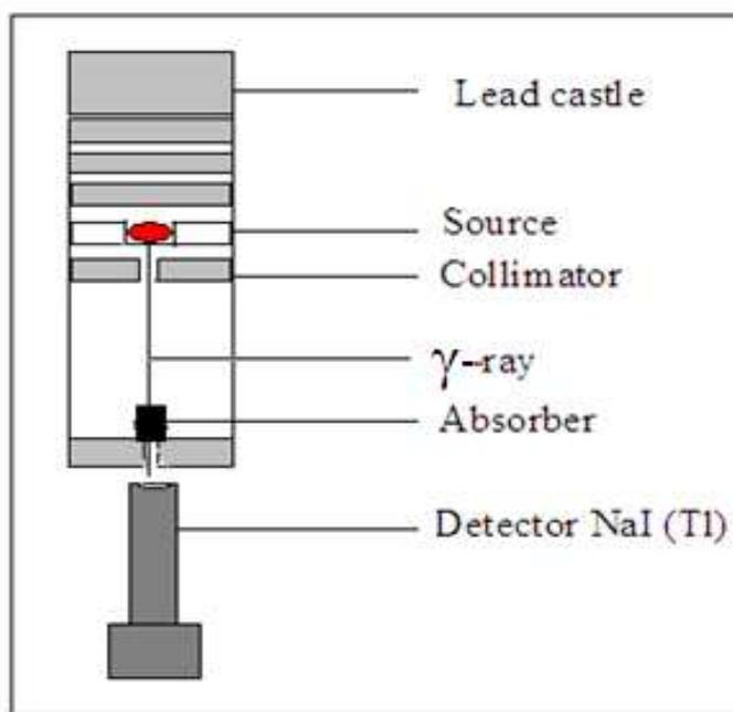
**Fig.1 Schematic Apparatus used for the measurement of  $\gamma$ -ray absorption coefficient**
