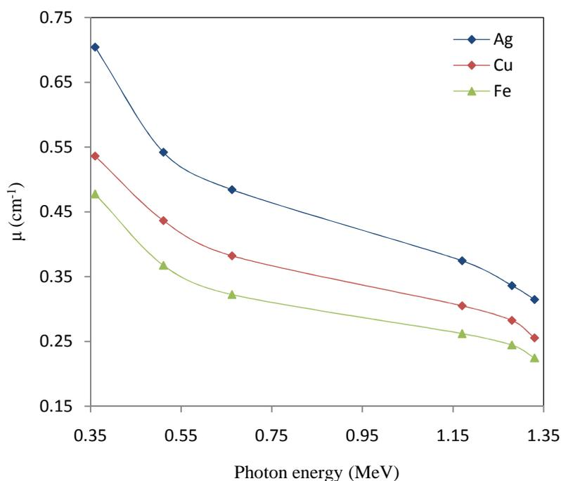
**Fig 3** Plots of photon attenuation coefficient ( $\mu$ ) v/s photon energy (MeV) for Ag, Cu and Fe (0.2 cm collimation)
