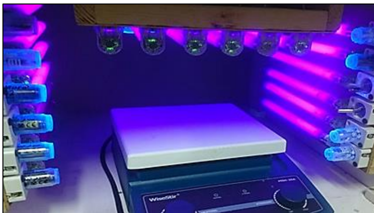
Figure 2: Schematic description of the homemade photoreactor that used in photocatalytic degradation
