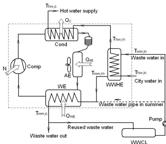
Figure 1. Diagram of flow chart and energy-exchanging of AWSHP water heater.
