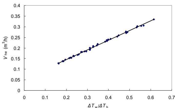
Figure 3. Relationship of  $V_{hw}$  and  $\Delta T_w/\Delta T_h$
