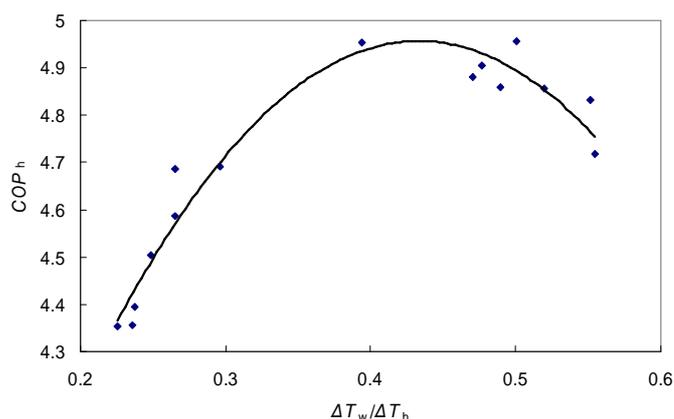
Figure 5. Relationship of  $COP_h$  and  $\Delta T_w/\Delta T_h$  in the AWSHP with reduced charged R22.
