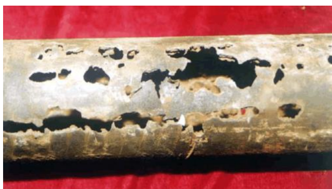
Fig.5: The tubing corrosion in sour gas reservoirs under coexistence of H 2 S and CO 2
