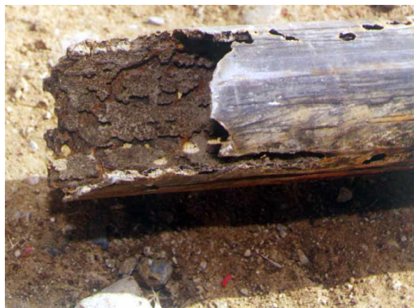
Fig.1: The tubing corrosion in a sour gas reservoir
