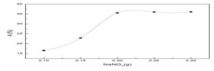
Fig.2.5 Relationship between the conversion rate and different amount of NaNO<sub>3</sub>
