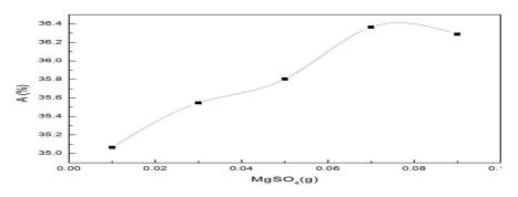
Fig. 2.6 Relationship between the conversion rate and addition of MgSO<sub>4</sub>
