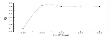
Fig.2.7 Relationship between the conversion rate and addition of K<sub>2</sub>HPO<sub>4</sub>
