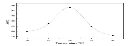
Fig.2.9 Relationship between the conversion rate and temperature
