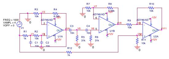
Fig. 1:The schematic diagram of filter circuit
