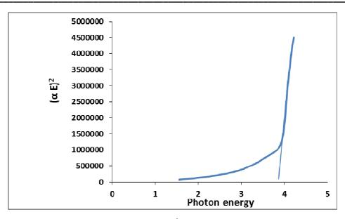
Fig.(3) The direct transition  $(\alpha h \upsilon)^2$  Vs. energy for PVC+1% ZnO
