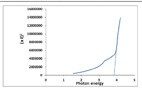
Fig.(5) The direct transition  $(\alpha h v)^2$  Vs. energy for PVC+10% ZnO
