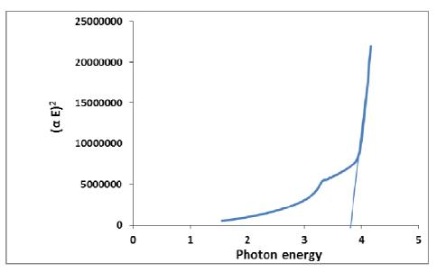
Fig.(6) The direct transition  $(\alpha hv)^2$  Vs. energy for PVC+20% ZnO
