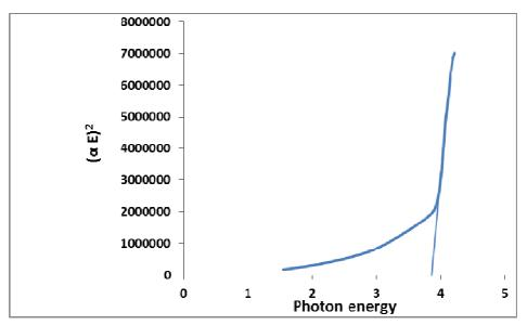
Fig.(4) The direct transition  $(\alpha hv)^2$  Vs. energy for PVC+5% ZnO
