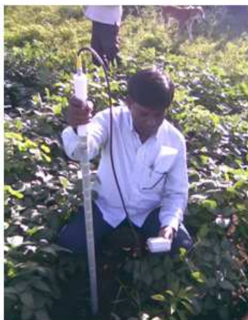
Figure 2. On field soil water content measurements with the help of profile probe at plot one.
