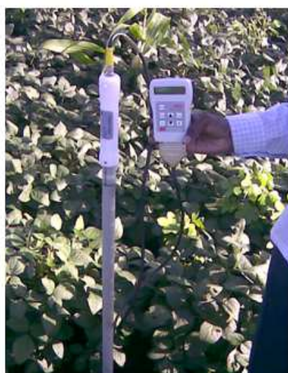
Figure 3. On field soil water content measurements with the help of profile probe at plot two.
