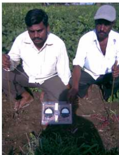
Figure 5. On field soil resistivity measurements with the help of profile probe at plot two
