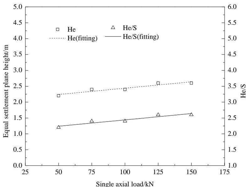
Figure 8. Effect of Single Axial Load on Equal Settlement Plane Height
