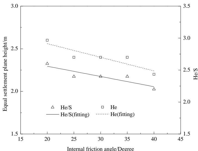
Figure 5. Effect of Internal Friction Angle of the Fill on Equal Settlement Plane Height
