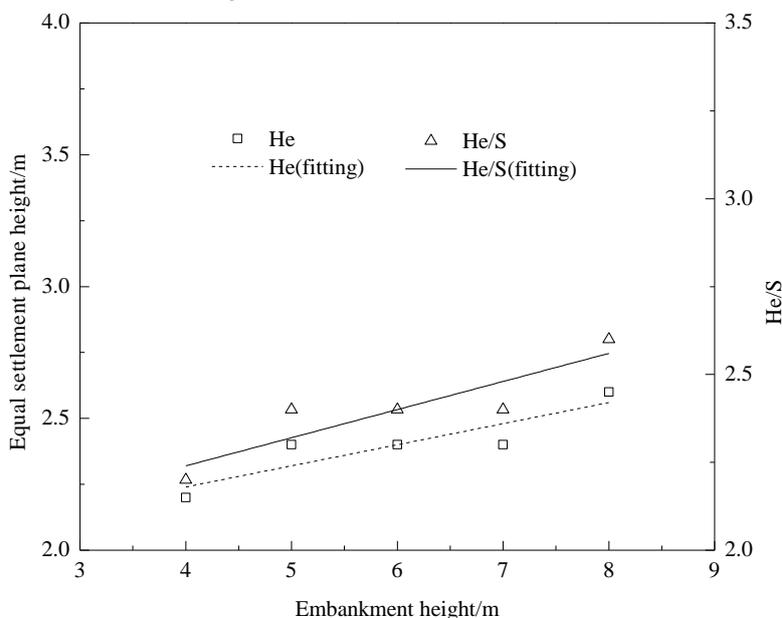
Figure 3. Effect of Embankment Height on Equal Settlement Plane Height
