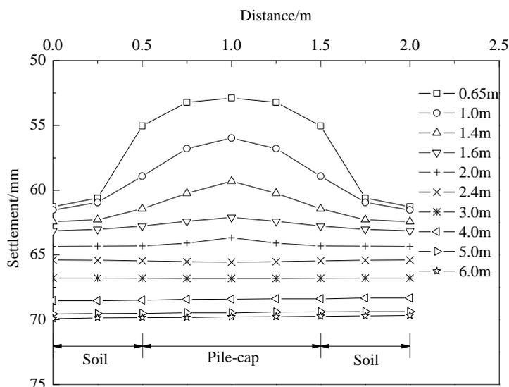
Figure 2. Settlements of the Embankment
