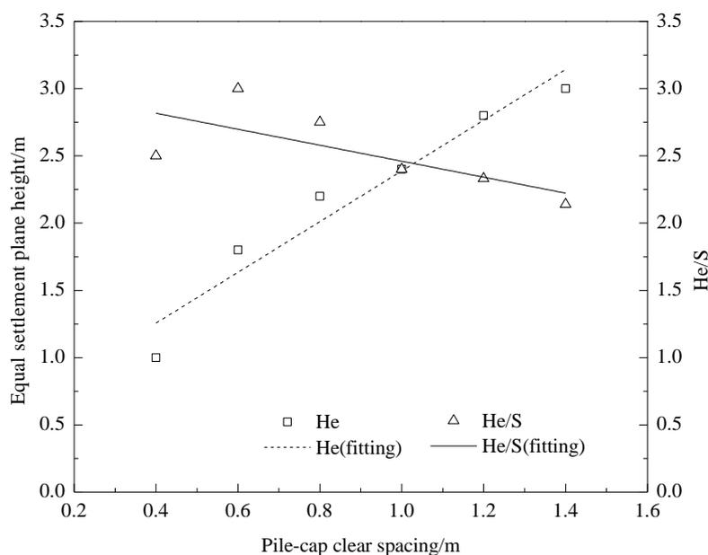
Figure 4. Effect of Pile-cap Clear Spacing on Equal Settlement Plane Height
