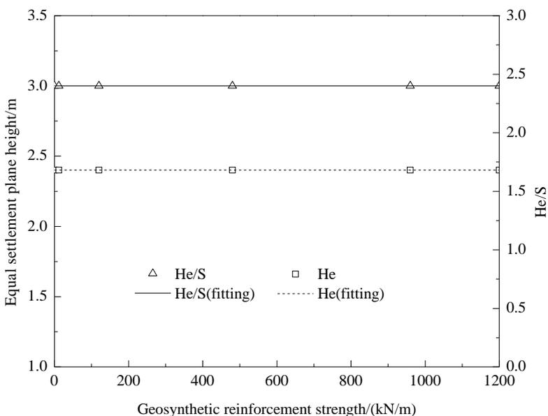
Figure 7. Effect of Geosynthetic Reinforcement Strength on Equal Settlement Plane Height
