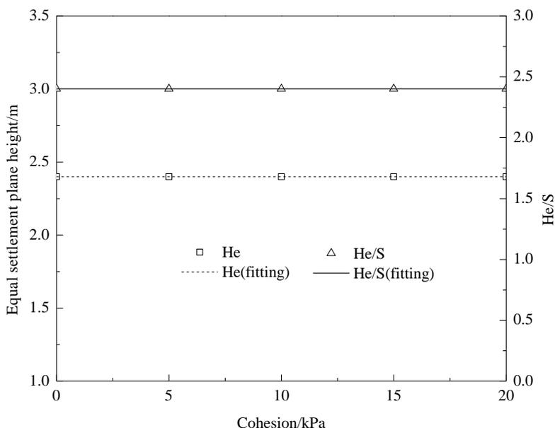
Figure 6. Effect of Cohesion of the Fill on Equal Settlement Plane Height
