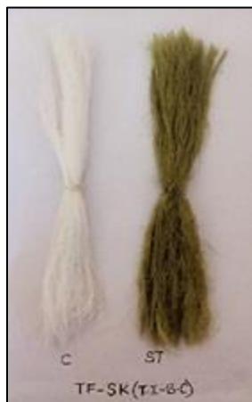
Figure 7: Dyeing of T.I-S.C meta mordanted silk yarn with Torenia sp flowers (50°C, pH 9, 30 min, ML-1:20)
