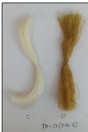
Figure 8: Dyeing of P.PT-B meta mordanted silk yarn with Torenia sp flowers (50°C, pH 9, 30 min, ML-1:20)
