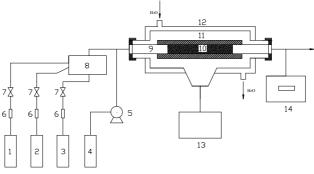
Fig. 1: Schematic diagram of microwave catalytic reactor
