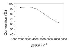
Fig. 6 Effects of GHSV on NO conversion
