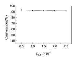
Fig. 4 Effects of NO feed concentration on NO conversion
