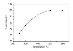
Fig. 3 Effects of reaction temperature on NO conversion
