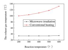
$\label{eq:comparison} \begin{array}{l} Fig.2 \ The \ comparison \ of \ exhaust \ gas \ temperatures \ under \ different \ reactor \ systems \ (Reaction \ conditions: \ molar \ fraction \ of \ O_2, \ 5.88\%; \ molar \ fractions \ of \ NO, \ 1\times10^{-3} \ and \ GHSV, \ 1920 \ h^{-1} \ and \ ambient \ temperature, \ 32^{\circ}C) \end{array}$
