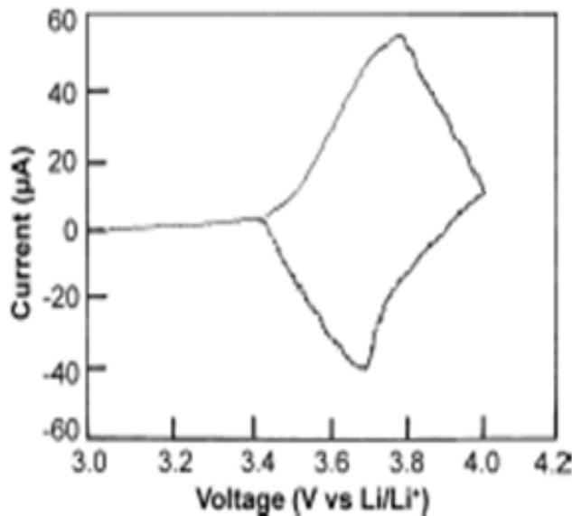
Figure 5: Cyclic Voltammogram of Li//LiNiO<sub>2</sub> cell deposited at 700 °C in pO<sub>2</sub> = 100 m Torr
