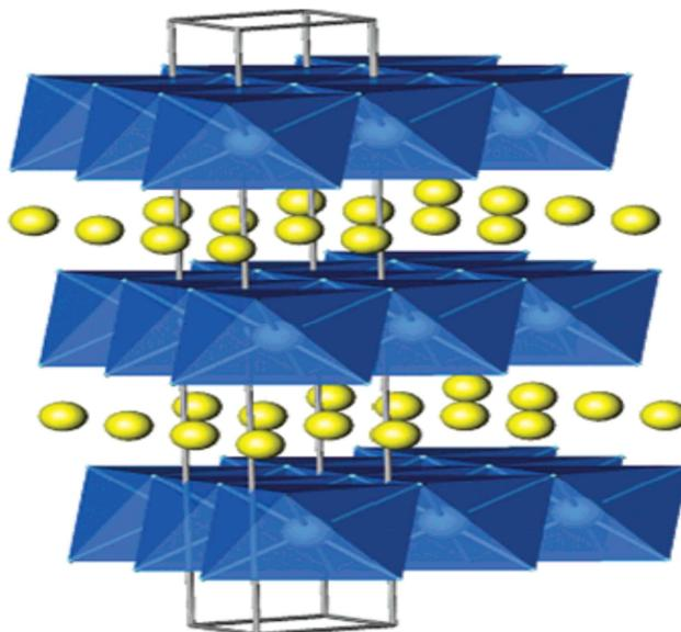
Figure 1: Layered structure of LiNiO<sub>2</sub> showing the lithium ions between the transition- metal oxide
