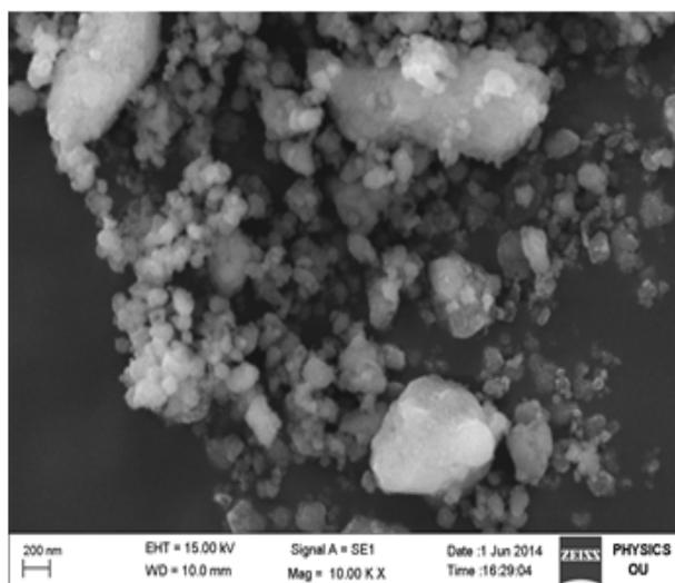
Figure 3: SEM image of LiNiO<sub>2</sub> thin film deposited at 700 °C in pO<sub>2</sub> = 100 m Torr
