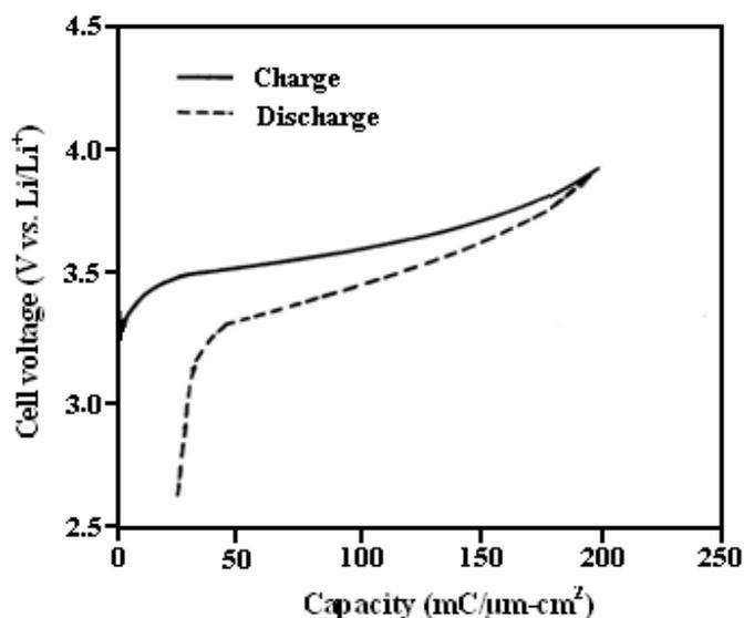
Figure 6: Charge - discharge profile of Li//LiNiO<sub>2</sub> cell
