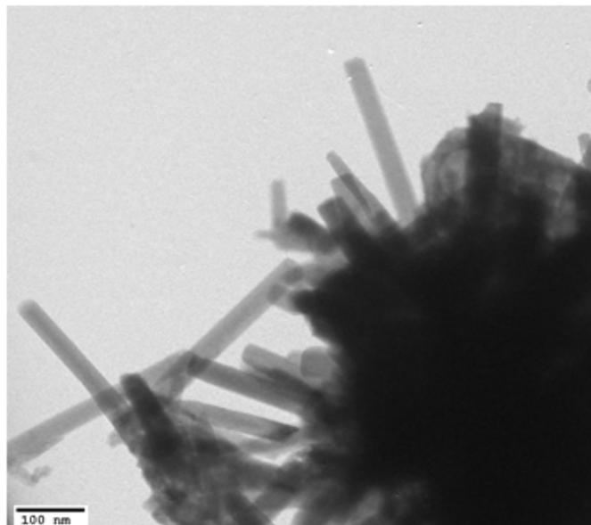
Figure 4: TEM image of LiNiO<sub>2</sub> thin film deposited at 700 °C in pO<sub>2</sub> = 100 m Torr
