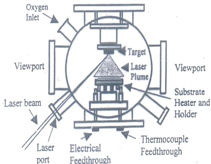
Figure 2 Schematic diagram of the pulsed laser deposition chamber
