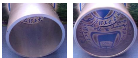
(a) Before finishing (b) After finishing Fig. 9. Comparison photos of aluminium hole surface
