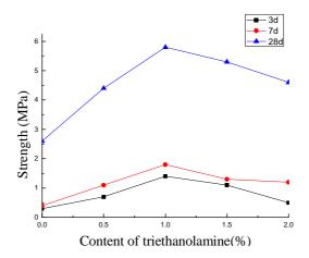
Fig.1 Effect of triethanolamine on compressive strength of steel slag-slag powder
