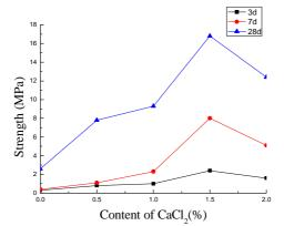
Fig.2 Effect of CaCl<sub>2</sub> on compressive strength of steel slag-slag powder
