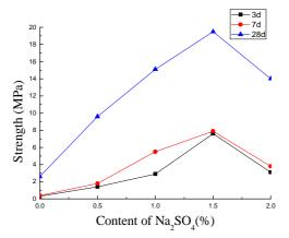
Fig.3 Effect of sodium sulfate on compressive strength of steel slag-slag powder
