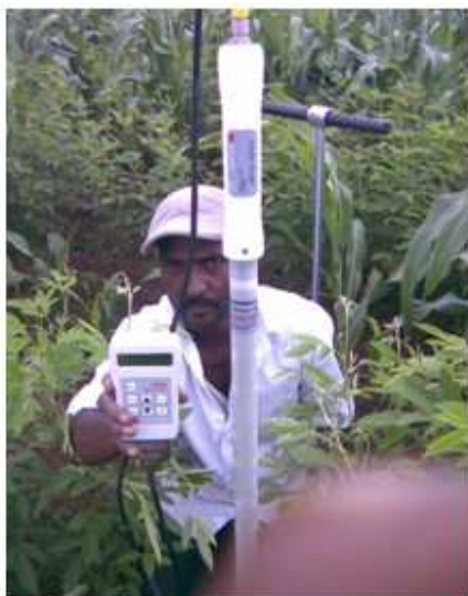
Fig. 3. On field soil water content measurement with the help of profile probe at test location two.
