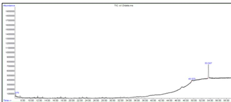
**Figure 2: GC-MS chromatogram of recovered crude extract which are hexadecanoic acid and octadecanoic acid were the major component formed during biodegradation of diesel oil**
