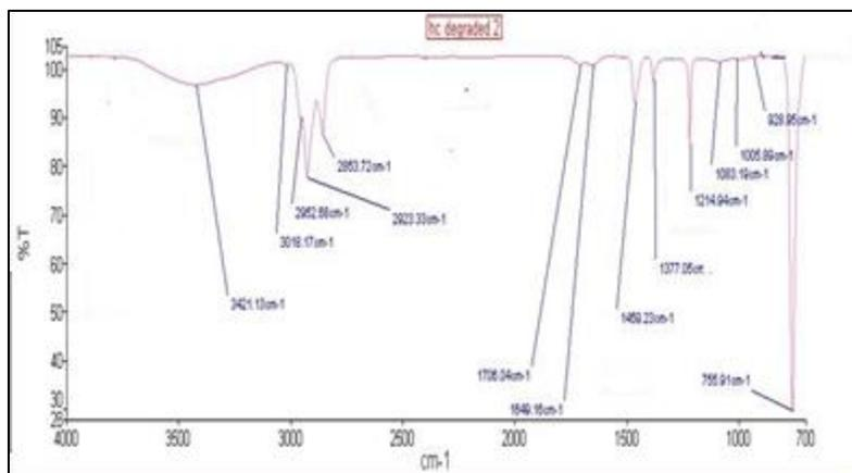
**Figure 1: FTIR analysis profile of degraded engine oil after 14 days of incubation**
