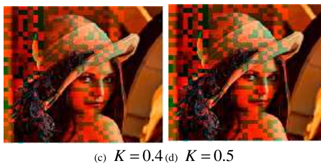
Fig. 5 :Changes of noise pattern under different embedding strength
