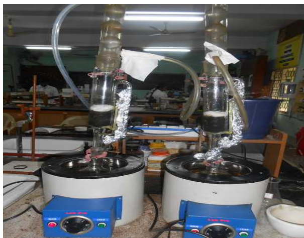
Fig.2: Soxhlet apparatus for the A.Malabarica leaves Extraction
