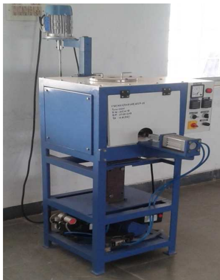
Figure 5 a) stir cast setup
