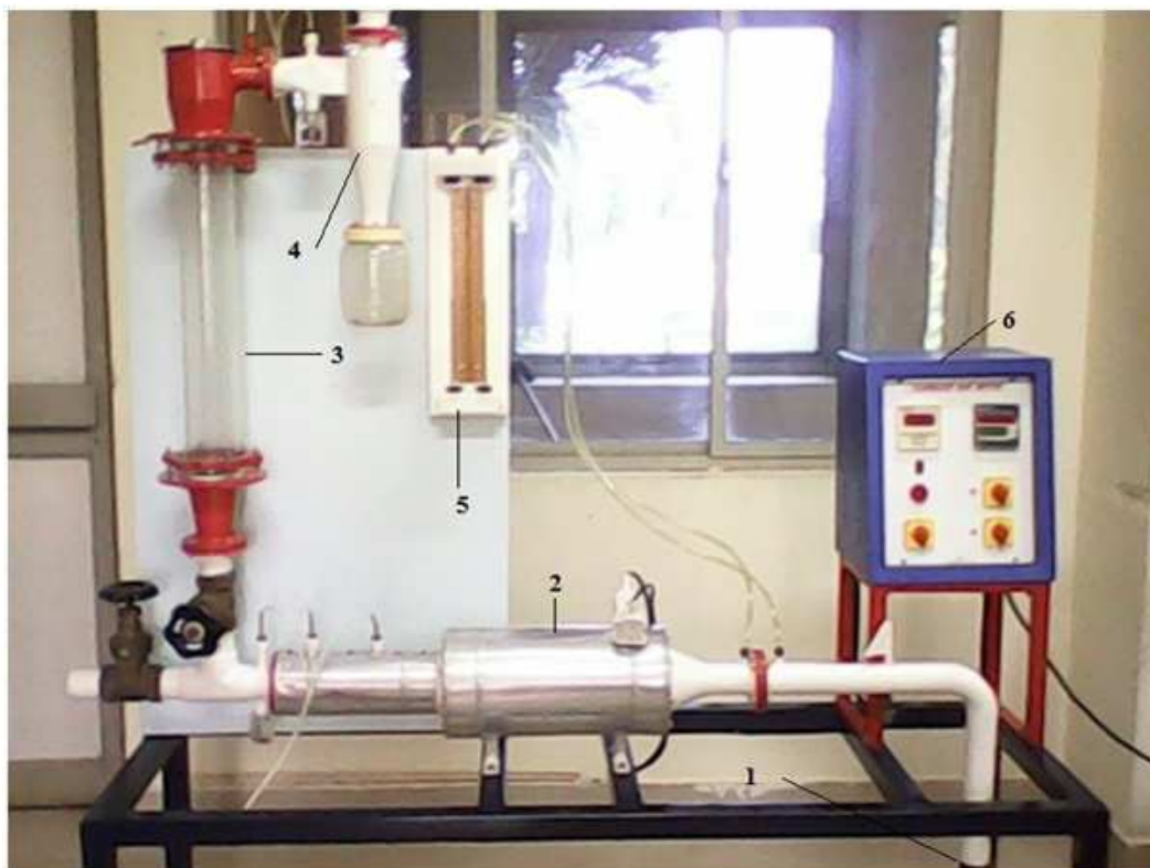
Fig. 1 Experimental set up of fluidised bed dryer 1-Blower, 2- Preheater, 3- Drying chamber, 4- Cyclone separator, 5- Water manometer, 6- Temperature indicator
