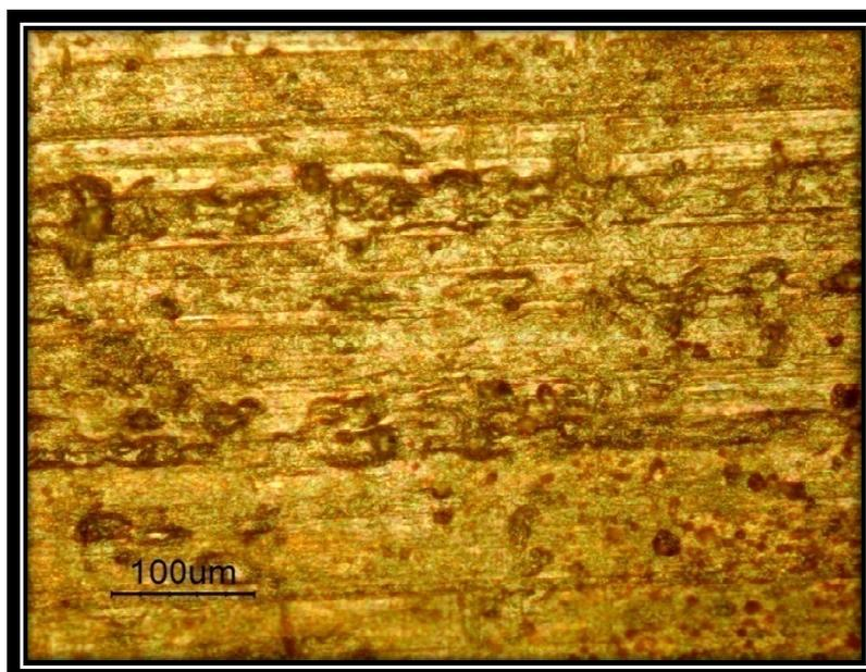
Figure (4): Optical Microscope images of (50 ppm) after potentiostatic test (general view (100µm))
