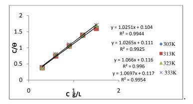
Figure 4 Langmuir adsorption isotherm in presence of leaves extract in 1M HCl
