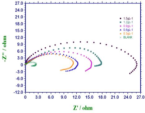
Figure 3 Impedance plots obtained in 1M HCl in various concentration of M. citrifolia L. at 303K
