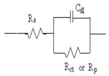
Figure 3 is a Randle circuit generally used to describe the aluminium acid interface model [0]
