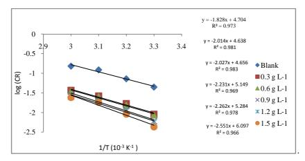
Figure 4 Arrhenius plot of the corrosion rate of the aluminium in 1M hydrochloric acid containing various concentrations of *M. citrifolia* L.
