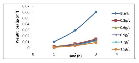
Figure 1. Weight loss versus immersion time for Al with different concentrations of leaves extract
