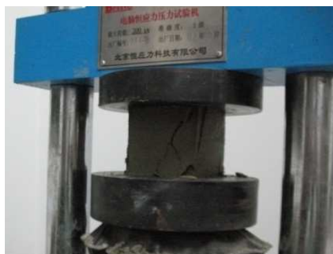
Figure 2: Uniaxial compressive strength test equipment
